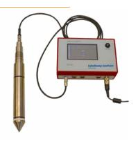
GeoExplorer is modern and versatile, and applies a database structure to store the recorded data. The latest version includes cloud technology, which allows remote monitoring of the CPT in real-time.
