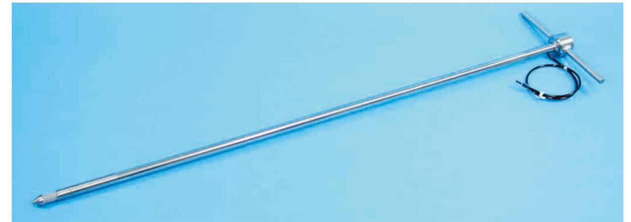
**DIK-5590** Cone penetrometer( easy operate soil hardness meter )
